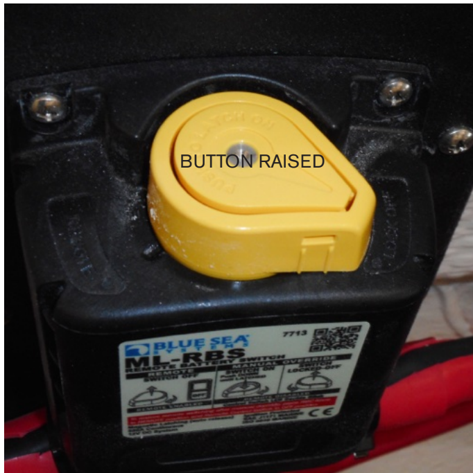
REMOTE BATTERY SWITCH- OFF POSITION
