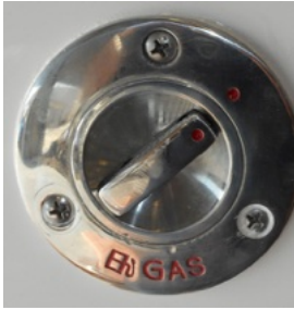
COMBO FUEL FILL/ INTERNAL VENT
