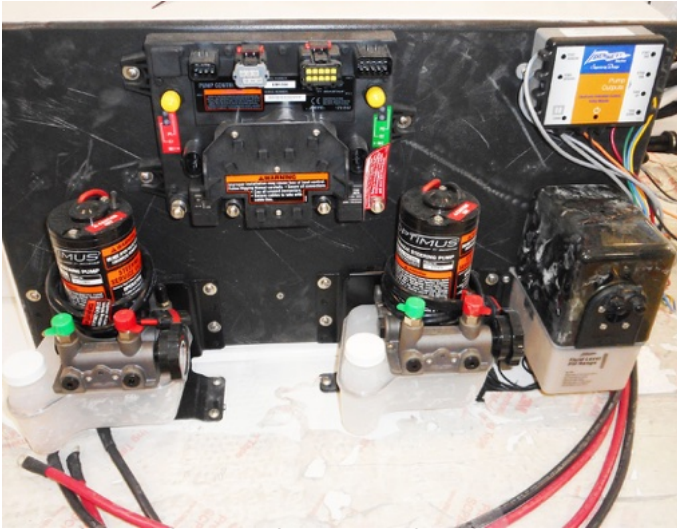
TYPICAL POWER STEERING BOARD
