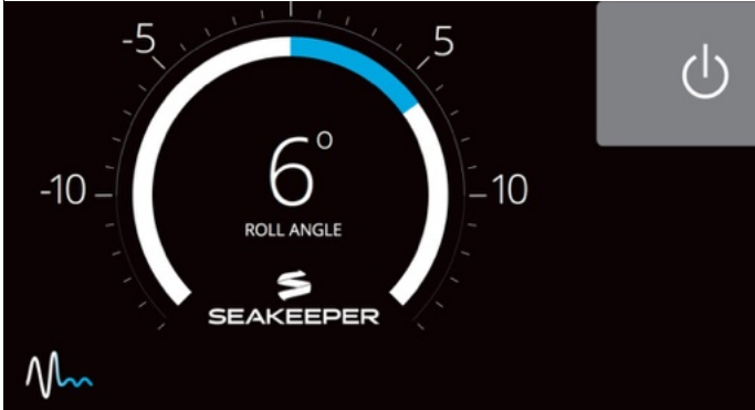
HOME SCREEN SHOWING POWER SWITCH W/TOUCH CONTROL
